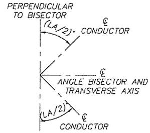
CONDUCTOR ATTACHMENT AXES
